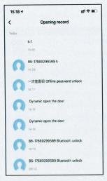
You can query the log in the door opening log, and the records are arranged in reverse order. The unlock ID that has been associated with the user name will directly display the corresponding user name, and the unlock ID that has not been associated with the name will display the specific unlock ID
